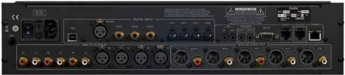
Analog inputs and outputs below; digital inputs and comms ports above.
