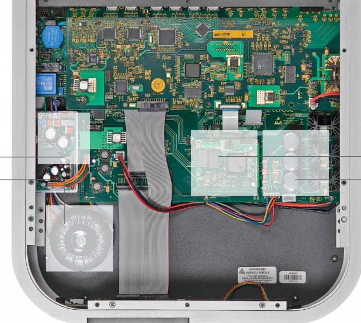
An independent low-voltage, high-current supply powers digital circuits.
