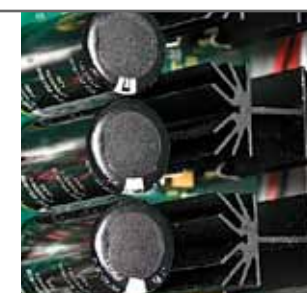
DC regulation for the analog supply is located near the front channel outputs on the right side of the chassis.
