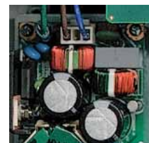
An independent low-voltage, high-current supply powers digital circuits.
