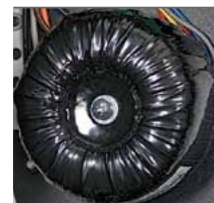
A custom designed low-noise toroidal transformer is used for the analog circuitry's linear power supply.
