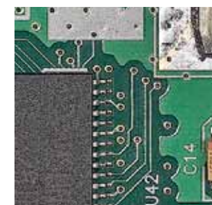
Digital Signal Processing is built onto a replaceable module.
